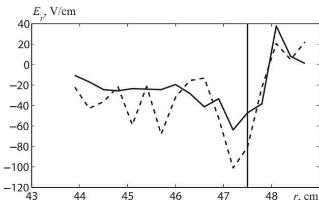
Fig. 5. Dependence of the radial electric field  $E_r$  on the radial coordinate  $r$ : Solid line corresponds to the Ohmic phase and dashed line to the DED phase of the TEXTOR discharge #111626. Vertical line shows the radial position of the limiter
