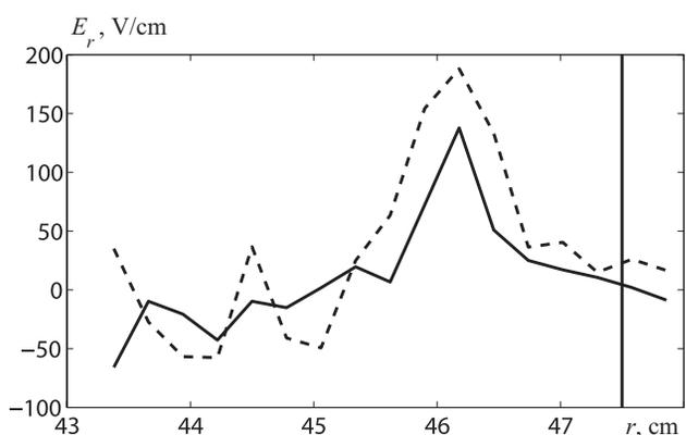
Fig. 3. Dependence of the radial electric field  $E_r$  on the radial coordinate  $r$ . Solid line corresponds to the Ohmic phase and dashed line to the biasing phase of the TEXTOR discharge #112172. Vertical line shows the radial position of the limiter
