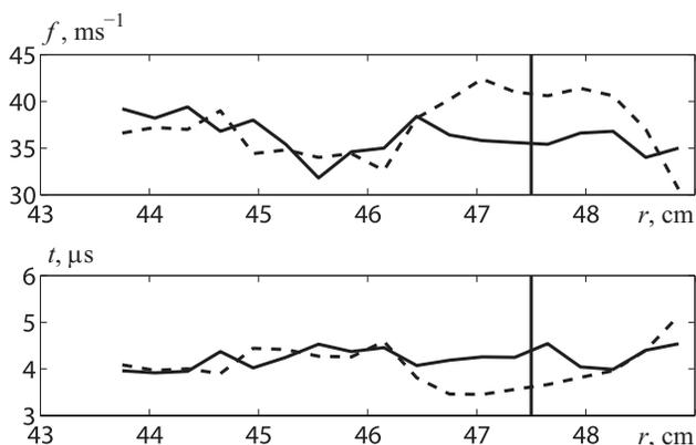
Fig. 4. Dependence of the  $I_{sat}$  average burst rate  $f$  (upper graph) and average burst duration  $t$  (lower graph) on the radial coordinate  $r$ . Solid lines correspond to the Ohmic phase and dashed lines to the DED phase of the TEXTOR discharge #111626. Vertical line shows the radial position of the limiter
