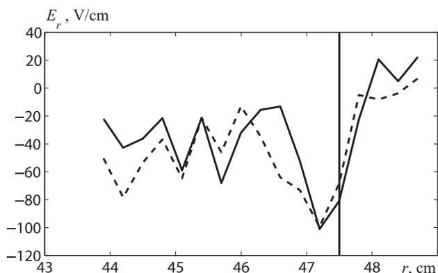
Fig. 10. Dependence of the radial electric field  $E_r$  on the radial coordinate  $r$  during DED phase of the TEXTOR discharge #111626. Solid line corresponds to the  $E_r$  calculated with contribution of temperature and dashed line to the one calculated without contribution of temperature. Vertical line shows the radial position of the limiter
