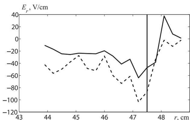
Fig. 9. Dependence of the radial electric field  $E_r$  on the radial coordinate  $r$  during Ohmic phase of the TEXTOR discharge #111626. Solid line corresponds to the  $E_r$  calculated with contribution of temperature and dashed line to the one calculated without contribution of temperature. Vertical line shows the radial position of the limiter
