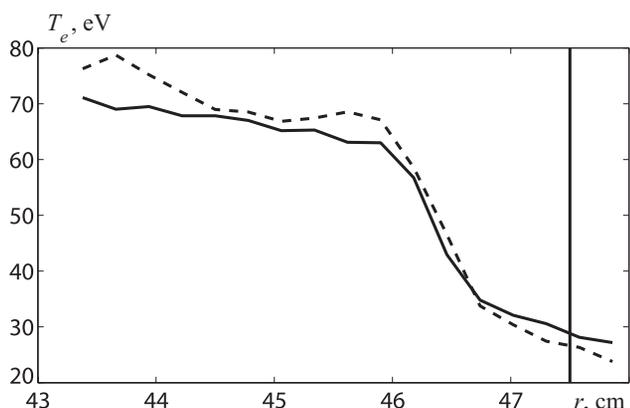
Fig. 8. Dependence of plasma electron temperature  $T_e$  on the radial coordinate  $r$ . Solid line corresponds to the Ohmic phase and dashed line to the biasing phase of the TEXTOR discharge #112172. Vertical line shows the radial position of the limiter
