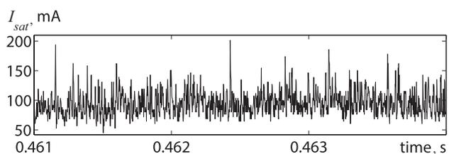
Fig. 1. Raw signal of ion saturation current  $I_{sat}$  measured at the edge of the TEXTOR tokamak
