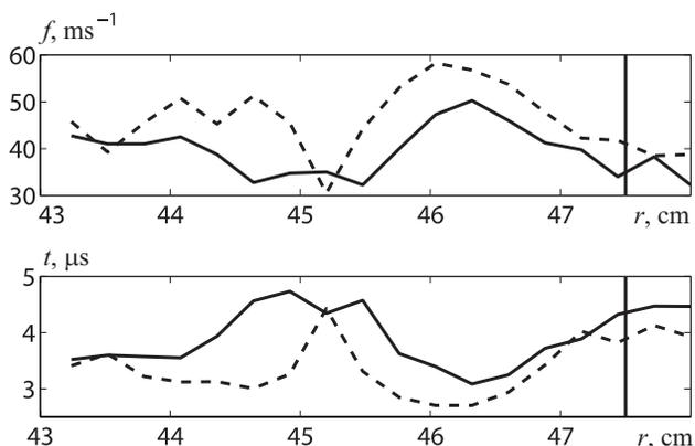
Fig. 2. Dependence of the  $I_{sat}$  average burst rate  $f$  (upper graph) and average burst duration  $t$  (lower graph) on the radial coordinate  $r$ . Solid lines correspond to the Ohmic phase and dashed lines to the biasing phase of the TEXTOR discharge #112172. Vertical line shows the radial position of the limiter
