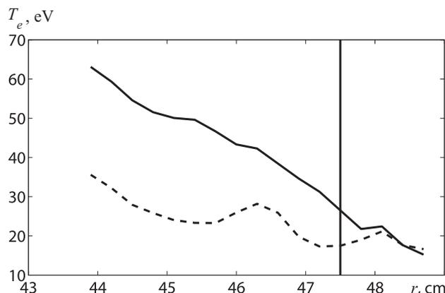
Fig. 11. Dependence of plasma electron temperature  $T_e$  on the radial coordinate  $r$ . Solid line corresponds to the Ohmic phase and dashed line to the DED phase of the TEXTOR discharge #111626. Vertical line shows the radial position of the limiter
