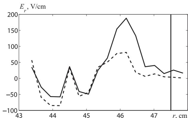
Fig. 7. Dependence of the radial electric field  $E_r$  on the radial coordinate  $r$  during biasing phase of the TEXTOR discharge #112172. Solid line corresponds to  $E_r$  calculated with contribution of temperature and dashed line to the one calculated without contribution of temperature. Vertical line shows the radial position of the limiter
