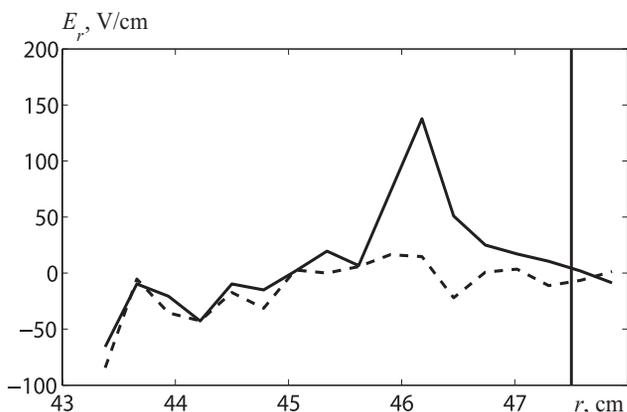
Fig. 6. Dependence of the radial electric field  $E_r$  on the radial coordinate  $r$  during Ohmic phase of the TEXTOR discharge #112172. Solid line corresponds to the  $E_r$  calculated with contribution of temperature and dashed line to the one calculated without contribution of temperature. Vertical line shows the radial position of the limiter
