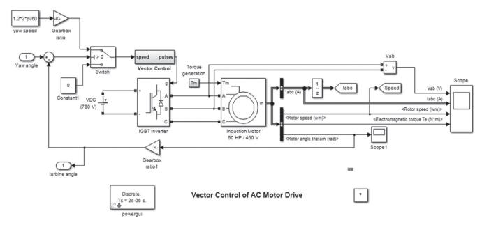
Fig. 7. Simulation model for yaw motor
