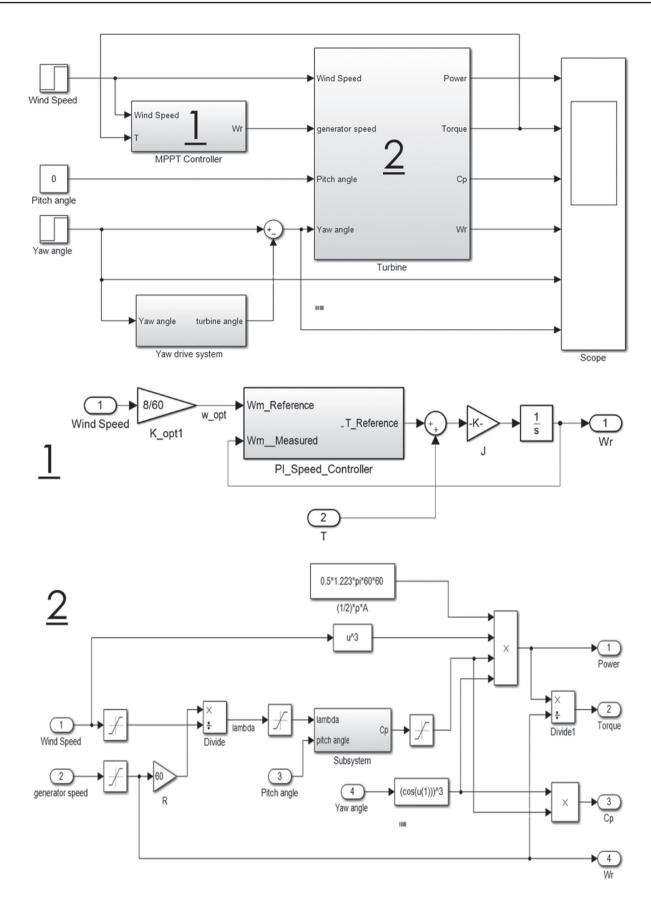
Fig. 4. Simulation modeling of the wind energy conversion system with contents of MPPT Controller (1) and Turbine (2)
