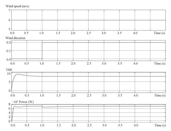
Fig. 9. The response of the WECS to a step change of the yaw angle 0 to 12° (just yaw system operate)
