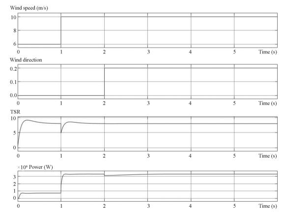
Fig. 11. Simulation results of the WECS operation with wind speed and direction change
