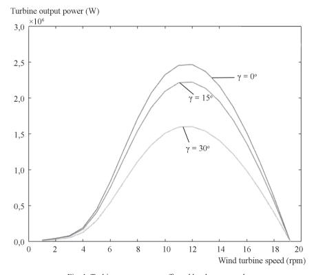
Fig. 1. Turbine output power affected by the yaw angle
