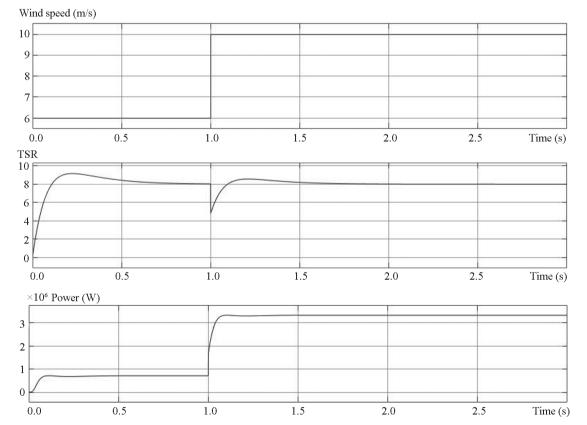
Fig. 8. The response of the WECS to a step change of the wind speed 6 to 10 m/s (just MPPT operate)
