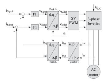
Fig. 5. Vector control of AC motor
