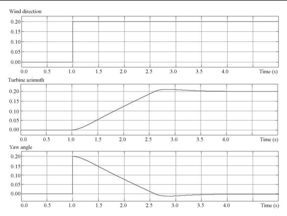
Fig. 10. Simulation results of yaw angle and turbine position
